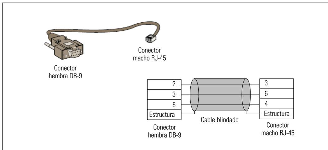
**Figura 37. Cable serial y patillaje DB-9/RJ-45**
