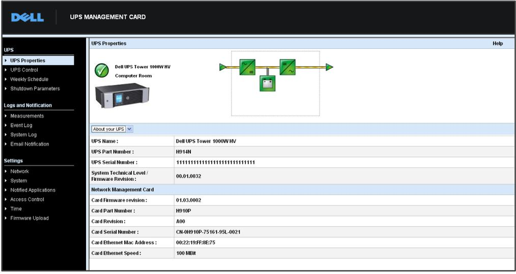
The screenshot displays the Dell UPS Management Card interface. On the left is a navigation menu with sections for UPS, Logs and Notification, and Settings. The main area is titled 'UPS Properties' and shows a 'Dell UPS Tower 1000W HV' in a 'Computer Room'. It includes a status indicator (green checkmark), a product image, and a simplified block diagram of the UPS system. Below this is a table with the following information:
